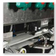
The fish doesn't need to be sorted before the vaccination. The system sorts the fish into three different weight classes, and can also separate fish that is too small, deformed or damaged.
